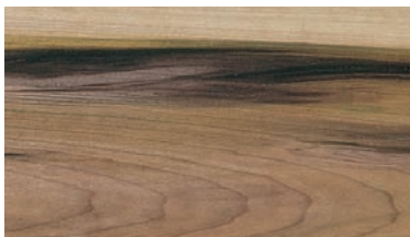
MINERAL STREAKS: Streaks of colour ranging from olive to blackish-brown, which typically follow the grain pattern.
