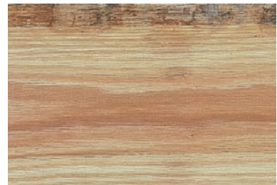
WANE: Bark or the lack of wood caused by the round nature of the tree or log.
