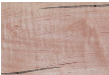
WORM HOLES: Holes in the wood ranging in size from \frac{1}{16} " to over \frac{1}{4} "
