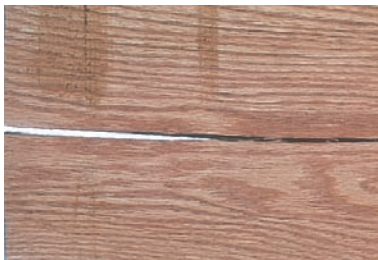
SPLIT: A lengthwise separation of the wood created as the wood dries. Shake is a separation between the annual growth rings.
