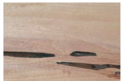
GRUB HOLES: Holes larger than \frac{1}{4} "
